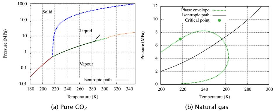
Figure 1: Isentropic depressurization from  $p = 12$  MPa,  $T = 293$  K.  $\text{CO}_2$  is in a dense liquid state until it reaches the saturation line and then the triple point, whereas the natural gas is in a dense gaseous state until it reaches the two-phase area. The Span–Wagner EOS has been used for  $\text{CO}_2$  and the Peng–Robinson EOS for natural gas. The natural gas composition is given in Table 1.
