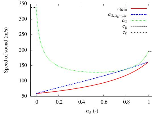
Figure 2: Speed of sound of pure CO<sub>2</sub> in the gas-liquid two-phase area as a function of gas volume fraction for various two-phase flow models.  $T = 250$  K, SW EOS. ‘hem’ denotes the homogeneous equilibrium model, ‘tf’ denotes the two-fluid model with no phase change and no slip, ‘tf  $\mu_g = \mu_l$ ’ is the two-fluid model with full chemical equilibrium and no slip, ‘g’ is gas and ‘l’ is liquid.
